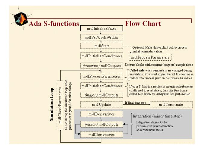
**Note** When interacting with Ada S-functions, the Simulink engine invokes only a subset of the callback methods that it invokes for C S-functions. The "Languages Supported" section of the reference page for each callback method specifies whether the engine invokes that callback when interacting with an Ada S-function.
