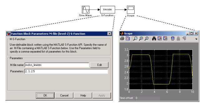
The model in this example incorporates the sample S-function
