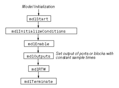
If the S-function resides in a conditionally executed subsystems, it is possible for the generated code to interleave calls to mdlInitializeConditions and mdlStart. Consider the following Simulink model sfcndemo\_enablesub.mdl.
