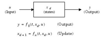
The dsfunc.c example implements a discrete state-space equation. The mdlOutputs method contains the output portion and the mdlUpdate method contains the update portion of the discrete state-space equation. To visualize
