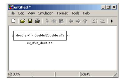
The following Simulink model demonstrates that the C MEX S-function produced by the Legacy Code Tool behaves like the C function doubleIt. In particular, the S-Function block named ex\_sfun\_doubleit returns the value of its floating-point input multiplied by two.
