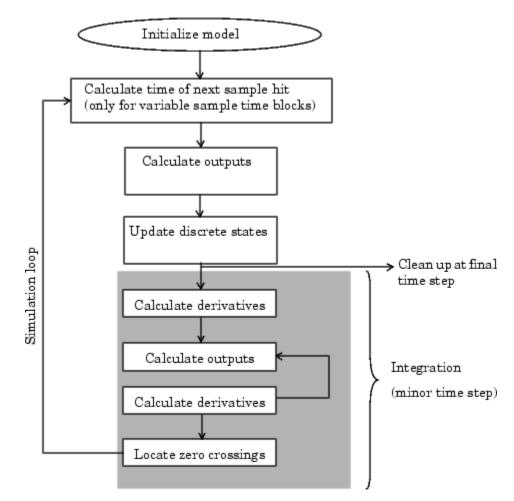
How the Simulink<sup>®</sup> Engine Performs Simulation
